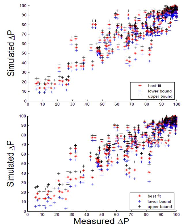
Fig. 4: Total predictive uncertainty intervals estimated with DREAM (left: log-likelihood function (LL); right: generalized likelihood function (GL) according to Schoups and Vrugt (2010)). Total predictive uncertainty intervals are given by the 2.5<sup>th</sup> and 97.5<sup>th</sup> percentiles of the posterior distribution of simulated  $\Delta P$  for each data point. Results are given for the run with the highest likelihood of the best parameter set out of ten trials.
