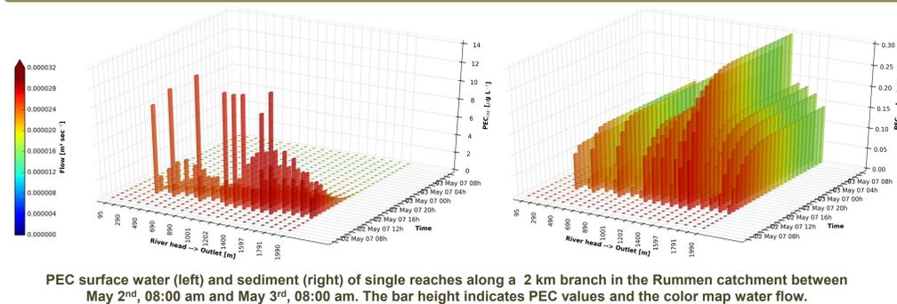
PEC surface water (left) and sediment (right) of single reaches along a 2 km branch in the Rummen catchment between May 2<sup>nd</sup>, 08:00 am and May 3<sup>rd</sup>, 08:00 am. The bar height indicates PEC values and the color map water flow.
