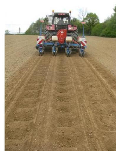
**Figure 1: Resulting pattern of micro-dams on the field.**
