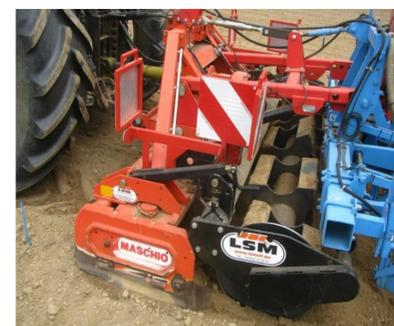
**Figure 2: Device for the installation of micro-dams (LSM, Belgium).**
