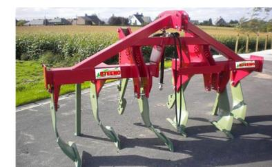
**Figure 3: Device to conduct the conservation tillage.**
