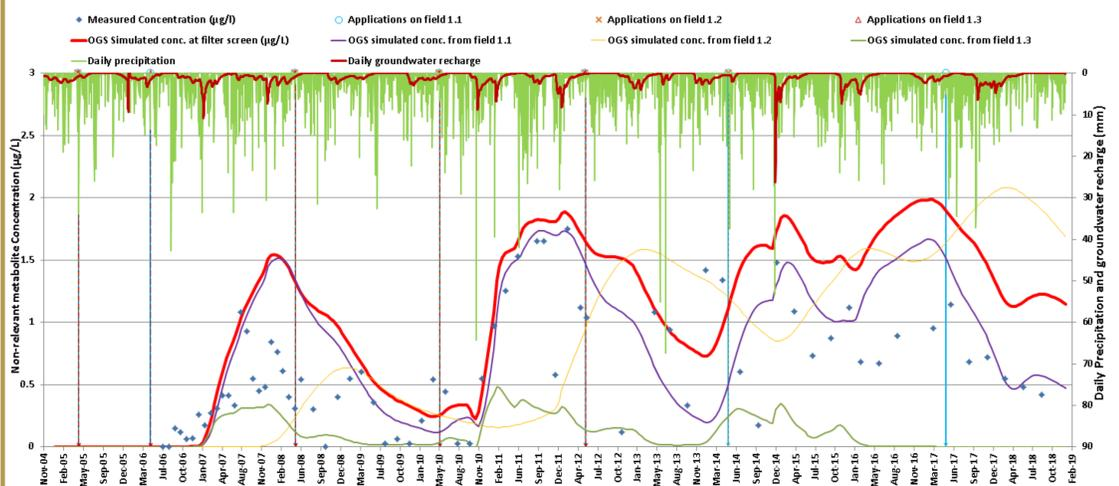
Figure 2: Comparisons of measured and simulated concentrations
