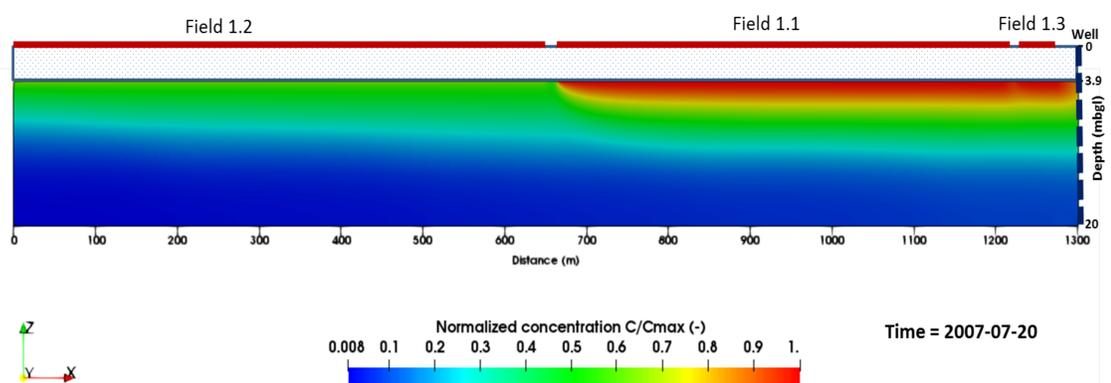
Figure 1: Illustration of model domain and distribution of normalized non-relevant metabolite concentration (direction of groundwater flow ==> from the left to the right)
